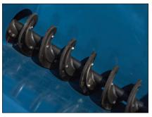
Virtually self-cleaning patented Talet® auger keeps grout flowing. The self-wiping polymer flighting discharges all material, eliminating build-up that could contaminate future batches. It moves varying aggregate sizes up to 1" without plugging or binding.
