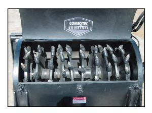
**Open-drum design** —The exclusive open drum design improves planer productivity by greatly reducing the power loss caused by the pics and drum passing through the already planed material. Standard planing drums lose power, particularly at depths below 1-1/2" because material is trapped between the pics and the drum. The open drum design overcomes this problem giving you increased productivity. The open drum shaft is supported on both ends by greasable heavy duty bearings.
